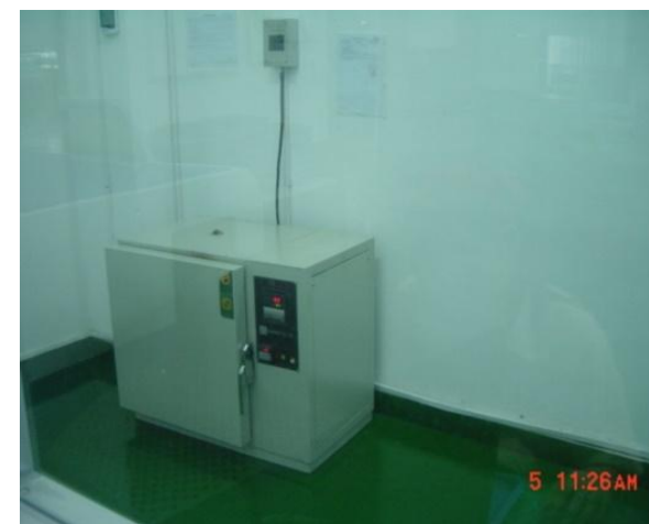
◀ Plastic performance and the product test high temperature machine 塑膠性能及產品測試高溫機
