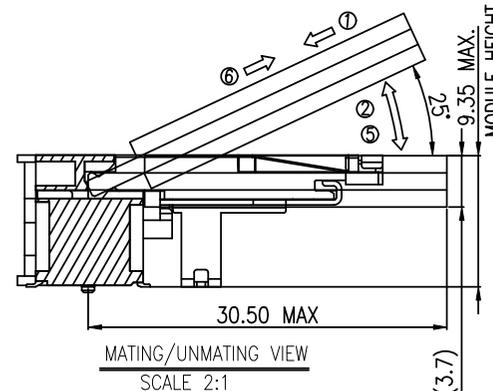
MATING: ① INSERTING(30°) → ② ROTATING → ③ FIXED
